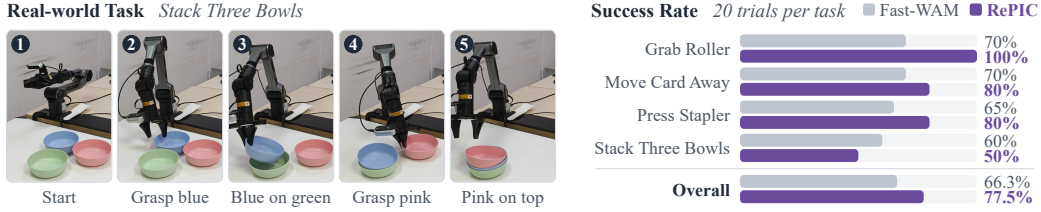
Figure 5: Real-world deployment. Left: a rollout of Stack Three Bowls on an Agilex Piper arm. Right: success rates over 20 trials per task for Fast-WAM and Fast-WAM with RePIC.
